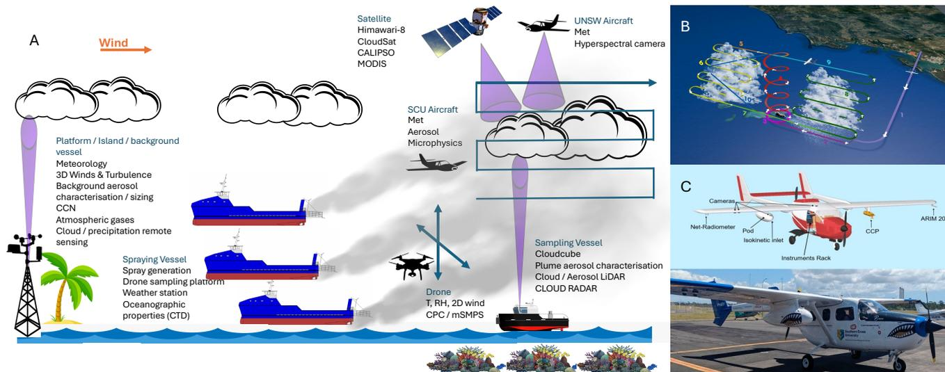
**Figure 4:** (A) The proposed major field campaign strategy. (B) Flight sampling strategy for aerosol and cloud physics sampling of upwind (background) and downwind (perturbed) cloud. (C) The SCU aircraft<sup>6</sup>.
