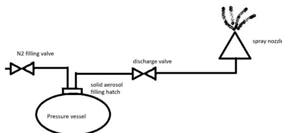
Figure 6. Example pressure vessel
