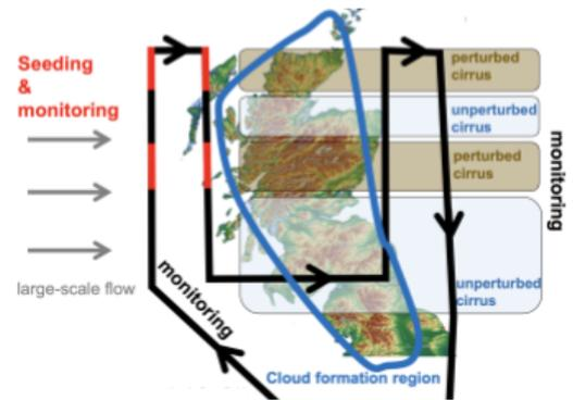
Figure 4. Schematic of the P3 seeding approach.
