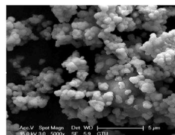
Figure 4. electron microscope image of a TiO<sub>2</sub> nanoparticle
