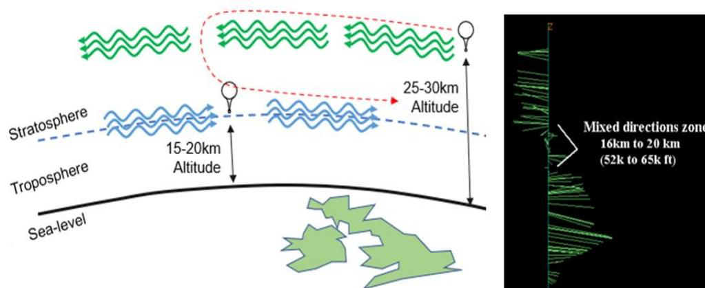
**Figure 5:** Navigation concept, in the light and variable winds of the lower stratosphere, just above the tropopause, a diversity of wind headings that rapidly change with small changes in altitude, can be selected by altitude controlling balloons to control drift direction and provide navigation.
