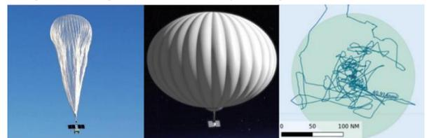
**Figure 3:** Example heavy category HAB, after launch (left), fully inflated in the stratosphere (middle), and example station-keeping performance over many days (right).
