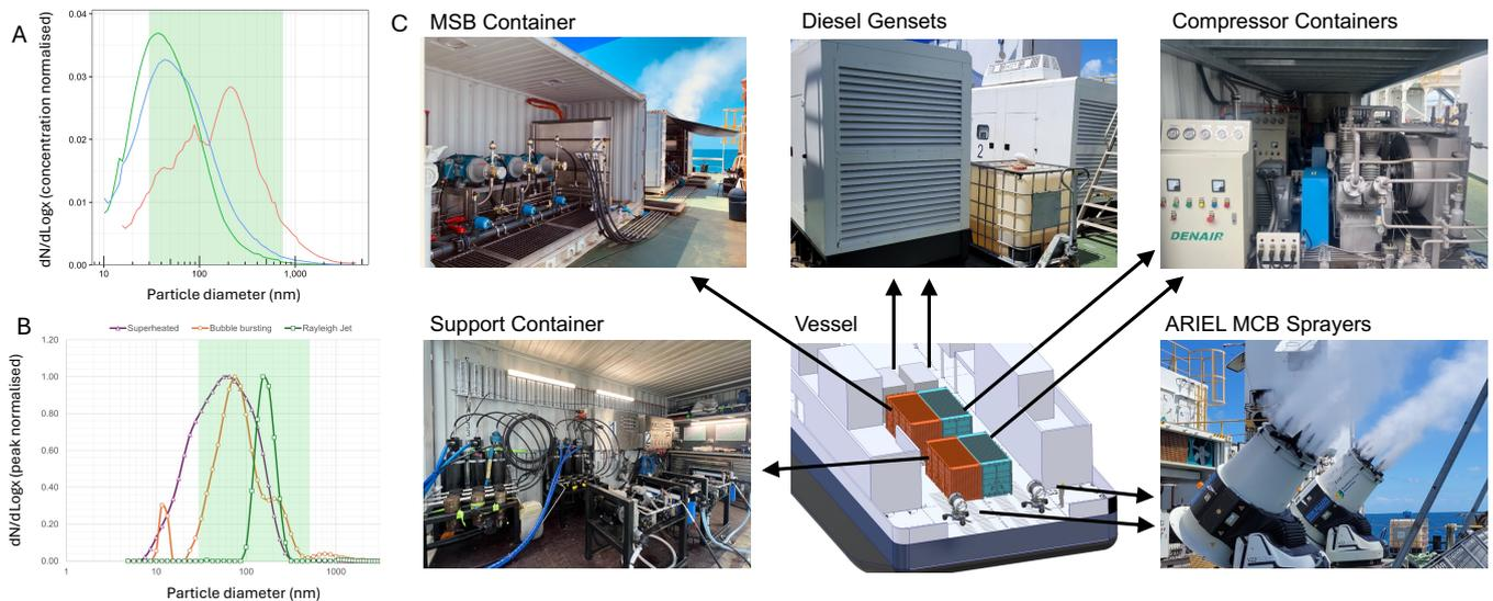
**Figure 3:** (A) Field measured size distributions for the 3 sprays currently produced by ARIEL. (B) Alternate spray technologies showing improved fraction in the target range (green shading). (C) ARIEL components.
