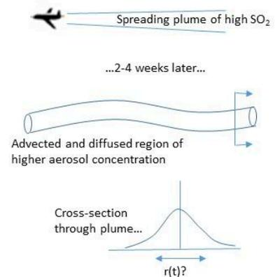
The initial plume of  $\text{SO}_2$  from the aircraft would gradually spread, advecting with the local winds, and diffusing (see sketch at right), but even after a few weeks would lead to a broad plume or tube of higher aerosol concentrations that is not at all close to uniformly mixed throughout the scale of a climate model grid cell (Newman et al., 2001).
