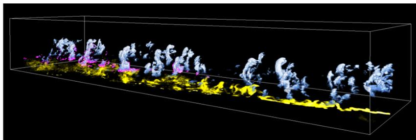
**Figure 2:** LES-LCM model results of a single MCB spraying vessel (at far right) in a shallow cumulus cloud field with wind right to left. White = cloud, Yellow = MCB aerosol, Magenta = aerosol impacted cloud.
